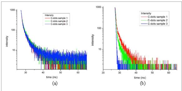
Figure 4. TRPL results of C-dots solutions synthesized from commercial granulated sugar using (a) hydrothermal method and (b) microwave.
