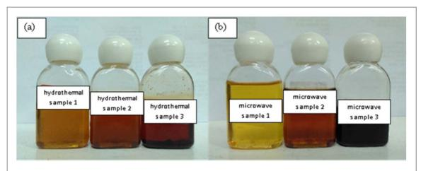
Figure 1. The C-dots solutions synthesized from commercial granulated sugar using (a) hydrothermal method and (b) microwave.
