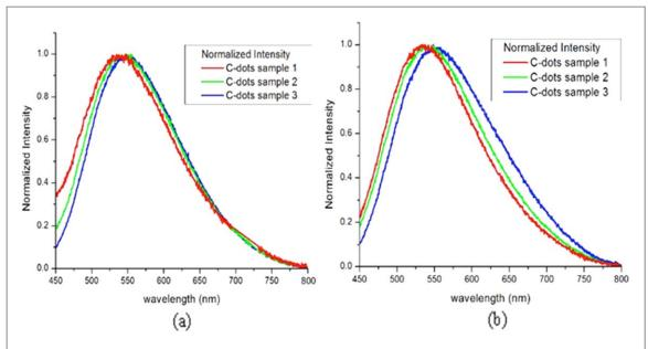
Figure 3. PL characterization results of the C-dots solutions synthesized from commercial granulated sugar using (a) hydrothermal method and (b) microwave.
