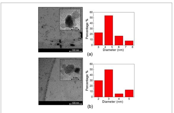
Figure 5. TEM images and diameter size distribution percentages of C-dots synthesized from commercial granulated sugar via (a) hydrothermal method and (b) microwave.
